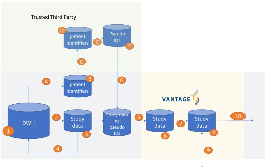
Figure 9. Flow chart of the data processing steps when analyzing a dataset with vantage6 when shared patient IDs are required.
